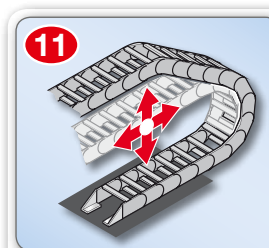
11 Installation option: Horizontal/vertical, combined
