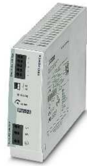
Power supply, 1 AC, 24 V DC, 10 A
