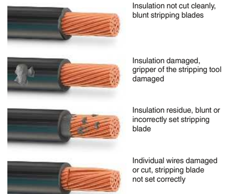
Cable stripped incorrectly in accordance with DIN IEC 60352-2
