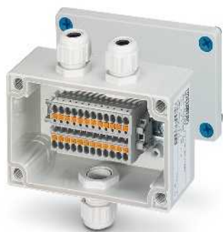
Terminal box with 12 2.5 mm 2 terminal blocks with Push-in connection technology
