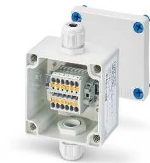
Terminal box with 6 2.5 mm 2 terminal blocks with Push-in connection technology
