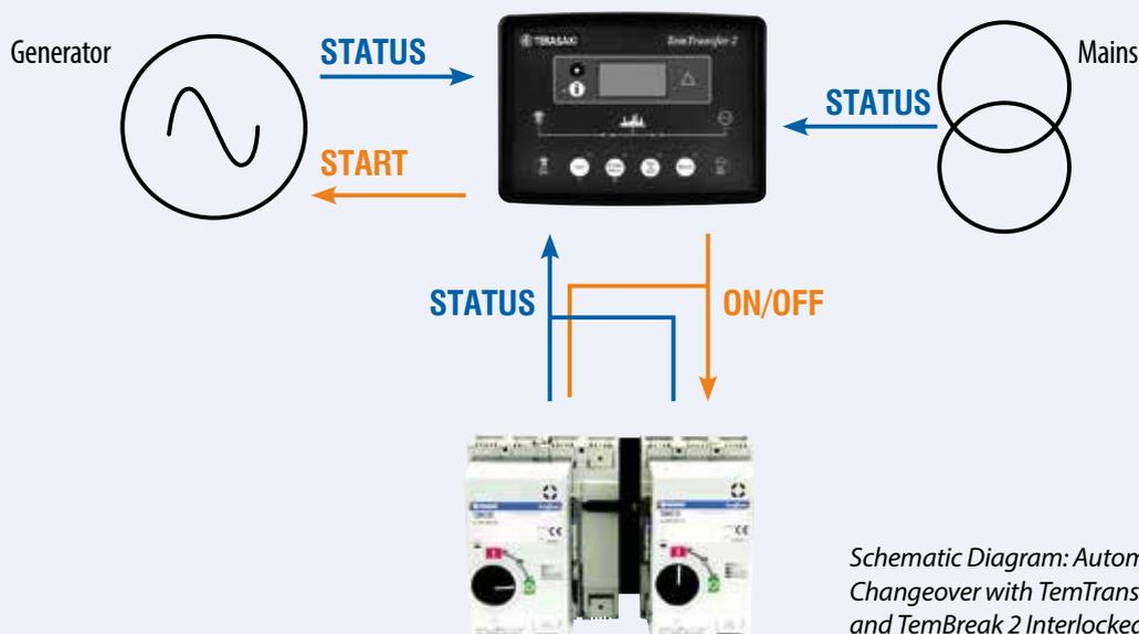
Schematic Diagram: Automatic Changeover with TemTransfer 2 and TemBreak 2 Interlocked MCCBs
