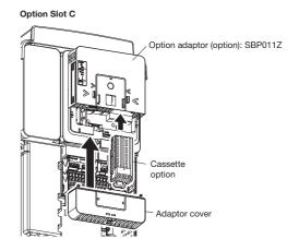
Note) The depth of the drive increases about 44mm when the option is mounted.
