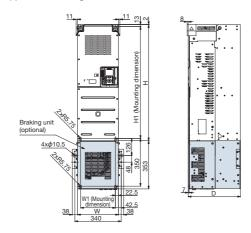
PB7-4200K is mechanically mounted on the left-hand side of the drive. Approx. mass 30kg
