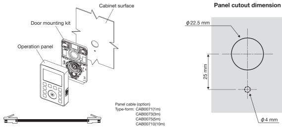
Note) Operation panel juts out about 26mm from the cabinet surface when the option is mounted on the cabinet surface.
