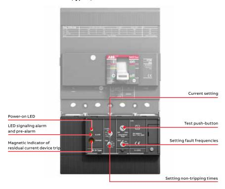
The RC residual current release type B, to be used in conjunction with the XT3 circuit-breaker, has the following features:
