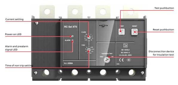
The fixed version of the RC Sel residual current release can easily be converted:
