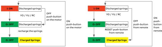
With the XT5 MOE and MOE-E and the XT6 MOE, it is possible to define some reset logic in order to charge the springs automatically once the circuit-breaker has tripped depending on the reset wiring diagram chosen. Three different options are available:
