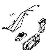
**35 - Main board + Sensors + cables for Trip unit M3 - Grey platform**
