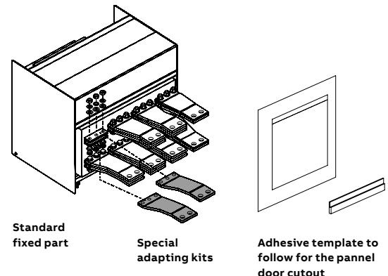
**Cradle in Cradle:** modifications are made to the fixed part of the old circuit-breaker that usually has bigger dimensions. A special fixed part for the new circuit-breaker is mounted into the old fixed part, so that the standard moving part of the new circuit-breaker can be easily racked in and out.
