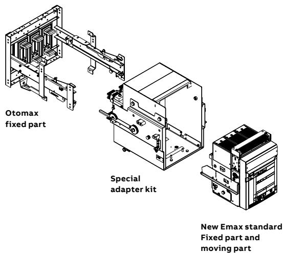
Before choosing any of the advanced solutions, it is necessary to verify that the fixed part is in good conditions: if it is irrevocably broken, it must be substituted. See our Fixed part checklist document (1SDH001279R0002).
