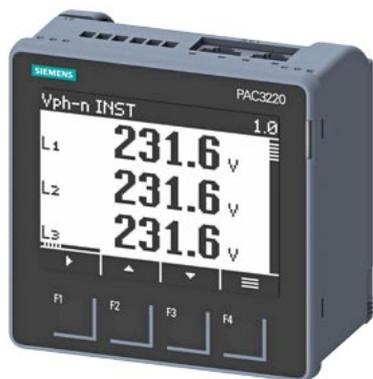
SENTRON PAC3220 LCD 96X96 mm Power Monitoring Device Control panel instrument for electrical values protocol: Modbus TCP with graphics display U rated input: 690/400V 45-65Hz IE rated input: X/1A oder X/5A AC Power supply: 100 ... 250 V +/-10 % AC/DC screw connections
