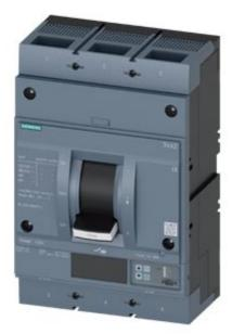
circuit breaker 3VA2 IEC frame 1000 breaking capacity class M Icu=55kA @ 415V 3-pole, line protection ETU550, LSI, In=800A overload protection Ir=320A...800A short-circuit protection Isd=0.6..10x In, Ii=1.5..12x In N conductor protection optionally with external current transformer, up to 160% nut keeper kit
