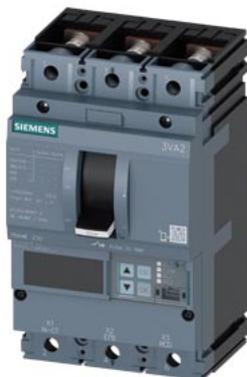
CIRCUIT BREAKER 3VA2 IEC FRAME 250 BREAKING CAPACITY CLASS M ICU=55KA @ 415 V 3-POLE, MOTOR PROTECTION ETU550M, LSI, In=200A OVERLOAD PROTECTION IR=80A ...200A SHORT CIRCUIT PROTECTION ISD=1,2... 15X IN,II=3...15X IN BUSBAR CONNECTION
