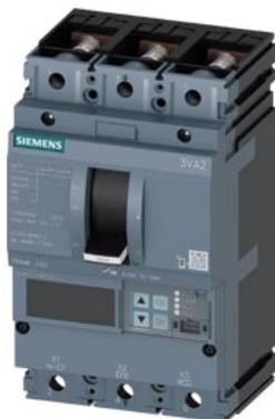
CIRCUIT BREAKER 3VA2 IEC FRAME 160 BREAKING CAPACITY CLASS M ICU=55KA @ 415 V 3-POLE, MOTOR PROTECTION ETU550M, LSI, In=25A OVERLOAD PROTECTION IR=10A ...25A SHORT CIRCUIT PROTECTION ISD=1,2... 15X IN,I=3...15X IN BUSBAR CONNECTION
