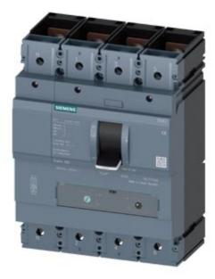
circuit breaker 3VA1 IEC frame 630 breaking capacity class M Icu=55kA @ 415V 4-pole, line protection TM240, ATAM, In=500A overload protection Ir=350A...500A short-circuit protection Ii=5...10 x In N conductor unprotected nut keeper kit
