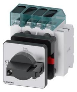
Load disconnector 3LD3, lu 63 A Main switch 3-pole + N Rated operating capacity at AC-23 A at 400V 22.0 kW Front plate mounting Basic switch with Central hole mounting 22.5mm Toggle drive black 48x48 mm with auxiliary switch 1OE + 1S
