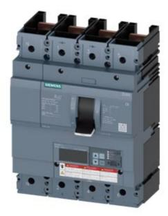
circuit breaker 3VA6 UL frame 600 breaking capacity class M 35kA @ 480V 4-pole, line protection ETU820, LI, In=600A overload protection Ir=240A...600A short-circuit protection Ii=1.5...9 x In without connection
