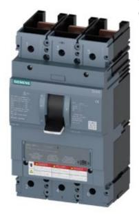
molded case switch 3VA6 UL frame 600 max. sh-circ breaking capacity 100kA @ 480V 3-pole, line protection MCS110, In=600A without overload protection self-protection li=9 x In without connection
