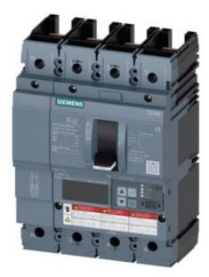
circuit breaker 3VA6 UL frame 150 breaking capacity class M 35kA @ 480V 4-pole, line protection ETU820, LI, In=100A overload protection Ir=40A...100A short-circuit protection Ii=1.5...12 x In without connection
