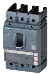
circuit breaker 3VA5 UL frame 250 breaking capacity class C 100kA @ 480V 2-pole, line protection TM210, FTFM, In=225A overload protection Ir=225A fixed short-circuit protection Ii=10 x In without connection
