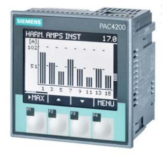
SENTRON, measuring device, 7KM PAC4200, LCD, L-L: 500 V, L-N: 289 V, 5 A, 3-phase, Modbus TCP, optional Modbus RTU / PROFINET / PROFIBUS / DI/DO, apparent/active/reactive energy / cos phi, harmonics: 3.-31., THD, class 0.2 acc. to IEC61557-12 or cl. 0.2S acc. to IEC62053-22, ext-low volt. pwr sup. unit DC, screw terminals
