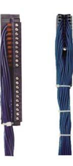
FRONT CONN. S7 SINGLE COR. 0.5QMM 5.0M Front connector for SIMATIC S7-300 20 pole (6ES7392-1AJ00-0AA0) with 20 single cores 0.5 mm2, Single cores H05V-K, Screw version VPE=1 unit L =  $5.0\ m$
