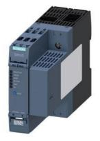
DC load monitoring relay for PROFINET, max. 1x63 A DC, max. 800 V Width: 45.0 mm Monitoring for violation of upper and lower limit of current, voltage and power; Energy consumption counter, energy recovery counter, switching cycle counter, operating hours counter, warning and alarm thresholds, automatic or manual reset, ON delay 0-999.0 sec, OFF delay 0-999.0 sec, automatic reclosing delay 0-999.0 sec Supply voltage: 24 V DC 1 changeover contact, screw terminal
