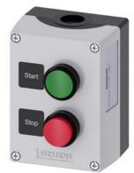
enclosure for command devices, 22 mm, round, enclosure material plastic, enclosure top part gray, 2 control points plastic, B=Pushbutton green, label: start, 1 NO, screw terminal, A=Pushbutton red, raised, label: Stop, 1 NC, screw terminal, floor mounting, 1xM20 each on top and bottom, Labels glued in
