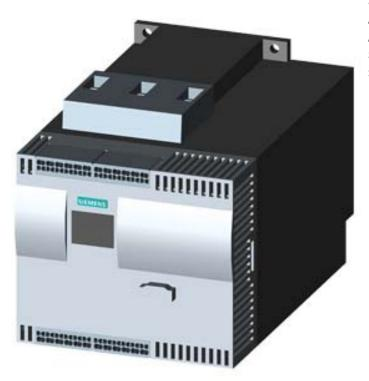
SIRIUS soft starter Values at 575 V, 50 °C standard: 26 A, 20 hp Inside-delta: 45 A, 40 hp 400-690 V AC, 115 V AC spring-type terminals !!! Phased-out product !!! Successor is SIRIUS 3RW5, Preferred successor type is >>3RW5524-3HA16<<
