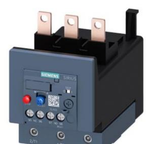
Overload relay 28...40 A Thermal For motor protection Size S3, Class 10 Contactor mounting Main circuit: Screw Auxiliary circuit: Screw Manual-Automatic-Reset
