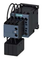
Capacitor contactor, AC-6b 12.5 kVAr, / 400 V 2 NC, 110 V DC 3-pole, Size S00 screw terminal
