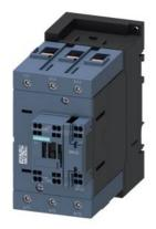
power contactor, AC-3 95 A, 45 kW / 400 V 1 NO + 1 NC, 110 V AC, 50 Hz 120 V/60 Hz 3-pole, 3 NO, Size S3 Spring-type terminal
