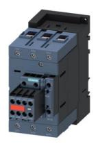
power contactor, AC-3 80 A, 37 kW / 400 V 2 NO + 2 NC, 230 V AC/50 Hz 3-pole, 3 NO, Size S3 screw terminal Captive auxiliary switch
