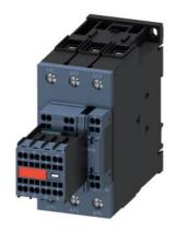
power contactor, AC-3 51 A, 22 kW / 400 V 2 NO + 2 NC, 24 V DC with varistor, 3-pole, size S2, spring-loaded terminal, captive auxiliary switch suitable for 2A PLC outputs
