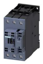
power contactor, AC-3 51 A, 22 kW / 400 V 1 NO + 1 NC, 400 V AC, 50 Hz 400-440 V, 60 Hz, 3-pole, size S2, spring-loaded terminal
