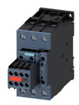
power contactor, AC-3 40 A, 18.5 kW / 400 V 2 NO + 2 NC, 24 V DC with varistor, 3-pole, Size S2, screw terminal Captive auxiliary switch Suitable for 2 A PLC outputs
