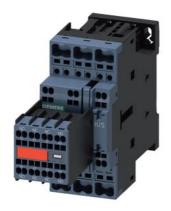
Power contactor, AC-3 38 A, 18.5 kW / 400 V 2 NO + 2 NC, 230 V AC 50/60 Hz, with inserted varistor 3-pole, Size S0 Spring type terminal Captive auxiliary switch
