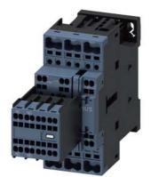
power contactor, AC-3 17 A, 7.5 kW / 400 V 2 NO + 2 NC, 400 V AC, 50 Hz, 3-pole, Size S0 Spring-type terminal Removable auxiliary switch
