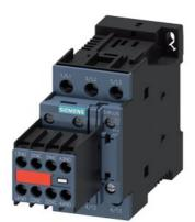
Power contactor, AC-3 17 A, 7.5 kW / 400 V 2 NO + 2 NC, 24 V DC, with inserted varistor 3-pole, Size S0 Screw terminal Captive auxiliary switch
