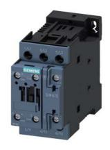
power contactor, AC-3 17 A, 7.5 kW / 400 V 1 NO + 1 NC, 24 V DC communication-capable, 3-pole, Size S0, screw terminal
