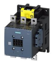
Contactor, AC-1, 500 A/690 V/40 °C, S10, 3-pole, 200-277 V AC/DC, F-PLC-IN with varistor, 2 NO+2 NC, Connection rail/ screw terminal
