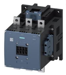
Power contactor, AC-3 500 A, 250 kW / 400 V AC (50-60 Hz) / DC 21-27.3 V UC Auxiliary contacts 2 NO + 2 NC 3-pole, size S12 Busbar connections Operating mechanism: solid-state with PLC interface 24 V DC screw terminals
