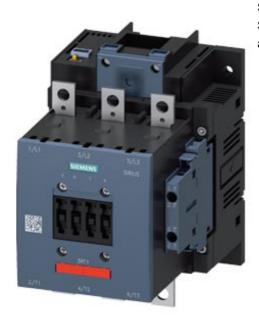
Power contactor, AC-3 185 A, 90 kW / 400 V AC (50-60 Hz) / DC operation UC 21-27, 3 V Auxiliary contacts 2 NO + 2 NC 3-pole, Size S6 Busbar connections Drive: electronic with PLC interface 24 V DC Screw terminal Auxiliary cont. lateral permanently mounted SUVA application
