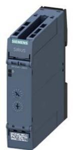
Timing relay, electronic OFF delay without control signal or smooth passing make contact non-volatile 7 time ranges 0.05...600 s 24 V AC/DC, 2 change-over contacts with LED, Spring-type terminal (push-in)
