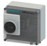
SIRIUS MCU motor starter Enclosure degree of protection IP55 plastic Communication without electromechanically switching Short-circuit protection with circuit breaker DOL starter Brake without Performance class 2.00 A Motor circuit breaker with bi-metal thermal Manual operation without Connection power M screw connection Standard product
