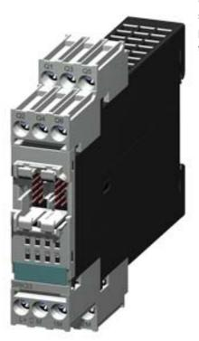
SIRIUS, Extension module 3RK33 for modular Safety system 3RK3 8 DO, 24 V DC/0.5 A Can be parameterized via MSS ES 22.5 mm overall width screw terminal without connection cable
