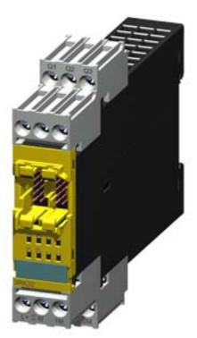
SIRIUS, Extension module 3RK32 for modular Safety system 3RK3 4 F-DO, 24 V DC/ 2 A Can be parameterized via MSS ES 22.5 mm overall width screw terminal Up to SIL3 (IEC 61508) Up to Performance Level E (ISO 13849-1) without connection cable
