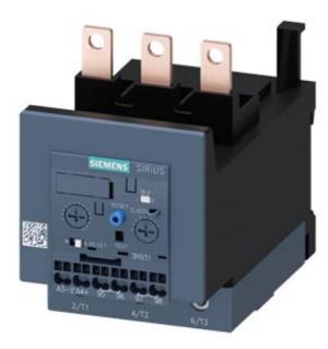
Overload relay 12.5...50 A Electronic For motor protection Size S3, Class 5E...30E Contactor mounting Main circuit: Screw Auxiliary circuit: Spring-type terminal Manual-Automatic-Reset
