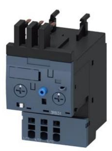
Overload relay 0.1...0.4 A Electronic For motor protection Size S00, Class 5...30 Contactor mounting Main circuit: Spring-type terminal Auxiliary circuit: Spring-type terminal Manual-Automatic-Reset Internal ground fault detection
