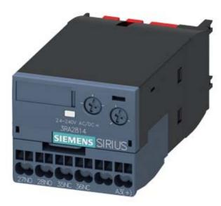
Solid-state time-delayed auxiliary switch OFF delay With control signal Relay 1 NC + 1 NO 24...240 V AC/DC Time range 0.05...100 s Can be snapped on at the front For 3RT2 S00-S3 contactors and 3RH2 S00 contactor relays Spring-type terminal Varistor for attenuation of the contactor coils integrated
