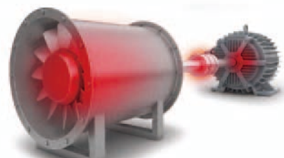
1. Abnormalities in load (blower fan) and rotary shaft 2. Effect on the current waveform of the motor
