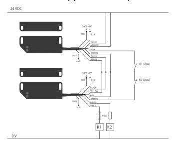
Two switches connected in series to give dual circuit safety outputs to machine contactors.
