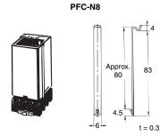
**Note:** PFC-N8 Mounting Bracket (provided with the Level Controller)
