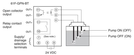
Note: 1. The part within the dotted-line box is for the 61F-GPN-BC (relay-output type) only.
