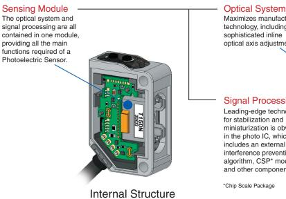
Maximizes manufacturing technology, including sophisticated inline optical axis adjustment.
