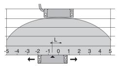
5 mm misalignment tolerance after setting
