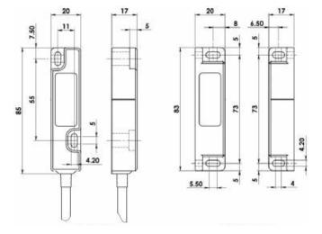
Wide Sensor (Sensor/Actuator) F3S-TGR-NWPR
