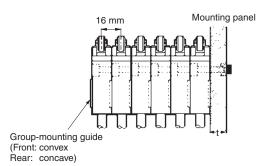
If the mounting panel is warped or has protruding parts, a malfunction may result. Make sure that the mounting panel is not warped and has even surfaces.
