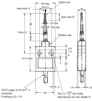
**Note: 1.** Operation is possible in any direction except in parallel to the axis -.
