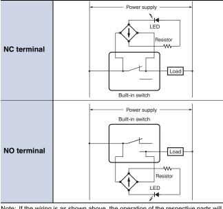
Note: If the wiring is as shown above, the operation of the respective parts will be as shown in the following table. The LED terminals are not wired when the Switch is delivered. Connect it as required.
